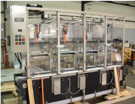
**ACID FILLER** – This new acid filler is becoming very popular. It can be used for initial fill, or top-off filling. It puts the right amount of acid into each cell, so that there is no need for a vacuum process after the fill. There is a 2, 3, or 4 head machine depending on your production needs. It uses templates to locate the fill nozzles, so change-overs are done very quickly.
