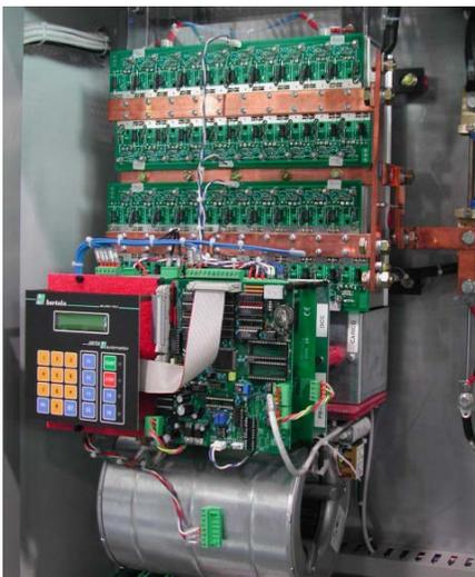
**DISCHARGER TESTER** - The modular discharger is an innovative product designed for 12V automotive batteries, end production line testing at a high current rate. The POWERMOS technology allows the ability to reduce the discharged current ripple down to zero, and better measures accuracy and fast transient response in comparison with the traditional discharge testers.
